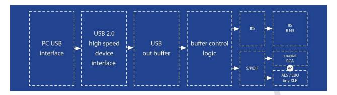
KingRex UC384 DDC designed by asynchronous. Inside the main chipset, it has buffer area for temporary storage stream data which helps to decrease the jitter and signal lose as well. Master clock generator is a classy 1ppm TCXO w/ proprietary driver lower jitter.
