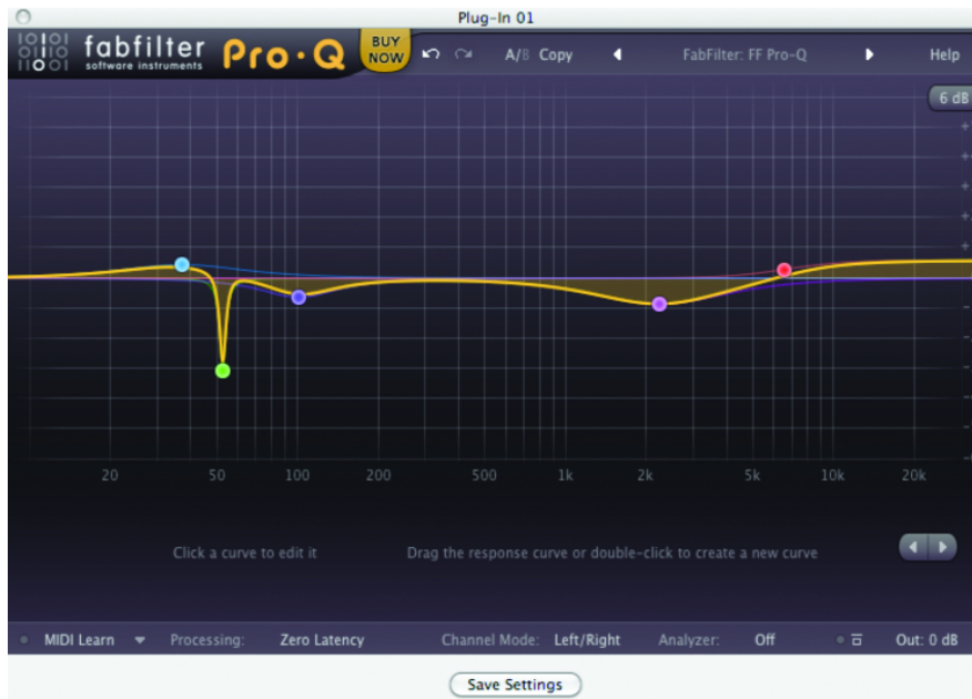
Third party (FabFilter Pro-Q) 24 band parametric equalizer plugin (plug-in is not included with Pure Music; shown for illustration)
